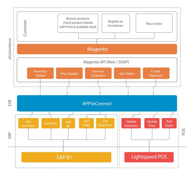
From the above architecture diagram, you can see our connector supports integration between any applications and uses full-fledged default APIs to integrate data between Magento with that of other external 3rd party apps.
